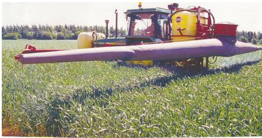
Figure 2. The PhytO3 Tech Crop Protection boom sprayer (Steffen, 2005b).
