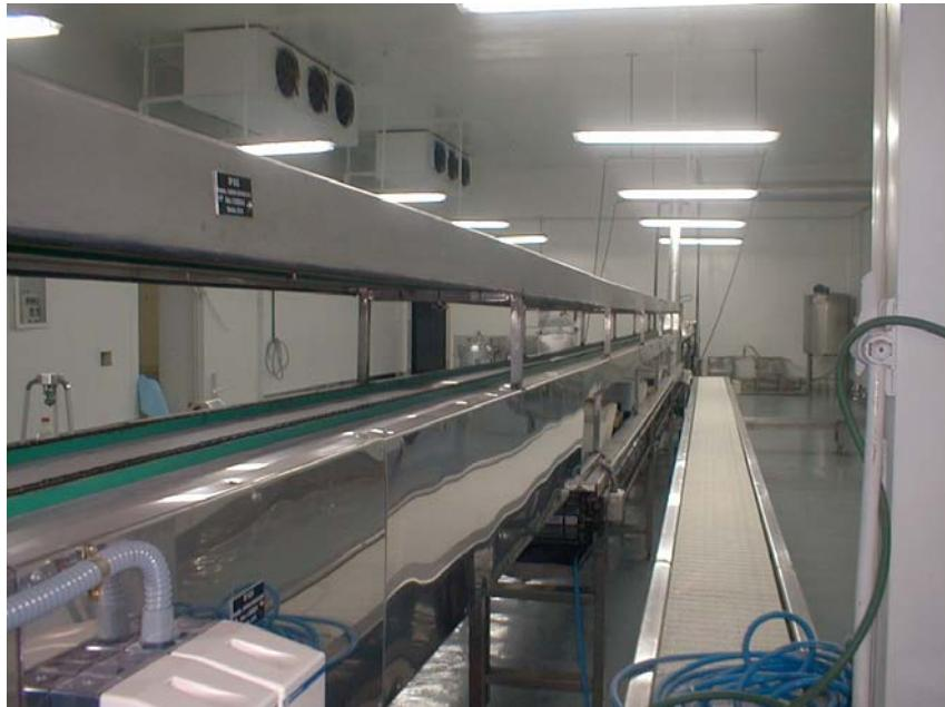
The ultra sound treatment is not only deadly to microbes but has also excellent cleaning properties to the surface of produce. This way it is possible to clean fresh cut delicate lettuce or baby leaves or bloody chickens without exposing them to abusing water agitation treatments and broccoli or cauliflowers and chickens are as well cleaned from inside. The produce is staying fresh crispy clean and without damages.
